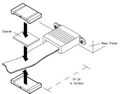
2 Insert the clamps onto the ends of the ferrites. The locking tab should fit cleanly in the ferrite grooves.
